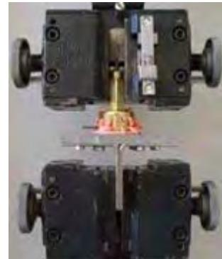
3 and 6 minutes after setting, the tensile force at failure was measured in a tensilometer (Zwick) at a crosshead speed of 500 mm/min. A non-adhesive group was used as control.
